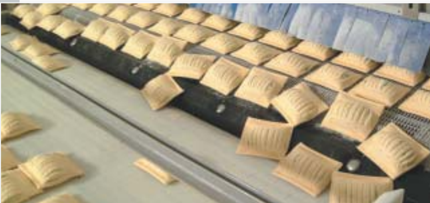
Eyelink belt used in freezing tunnel at Bakkersland, Hoogeveen, Holland.
