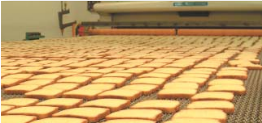
Spiral wirelink belt in furnace at Bolletje, Almelo, Holland.
