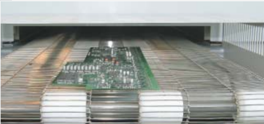
Wire mesh belt used in soldering furnace.
